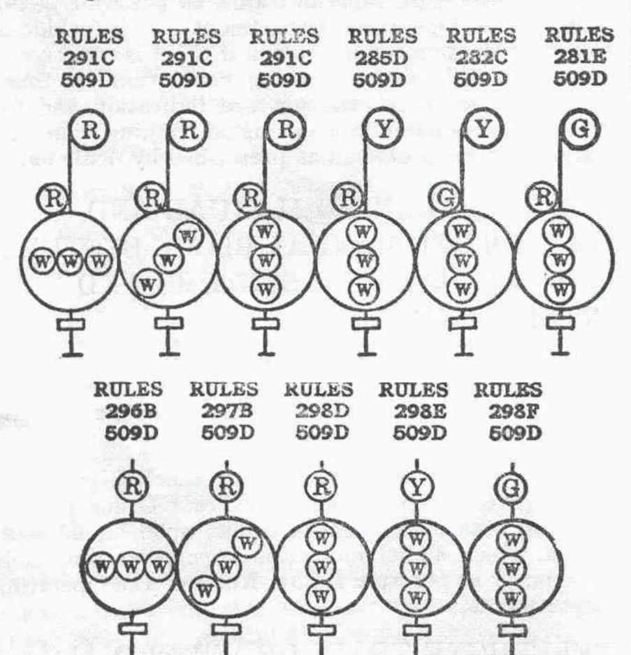
Where position light telephone train order signals are in service Rules 509b, 509c and 509d will be observed the same as where other types of signals are in use.
