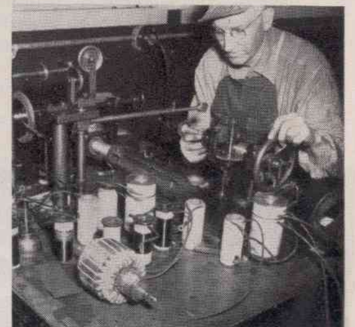
ABOVE: Relays are tested, adjusted and sealed in a dustproof room at the Meadville signal shop. In right foreground is bench where code units are checked.
