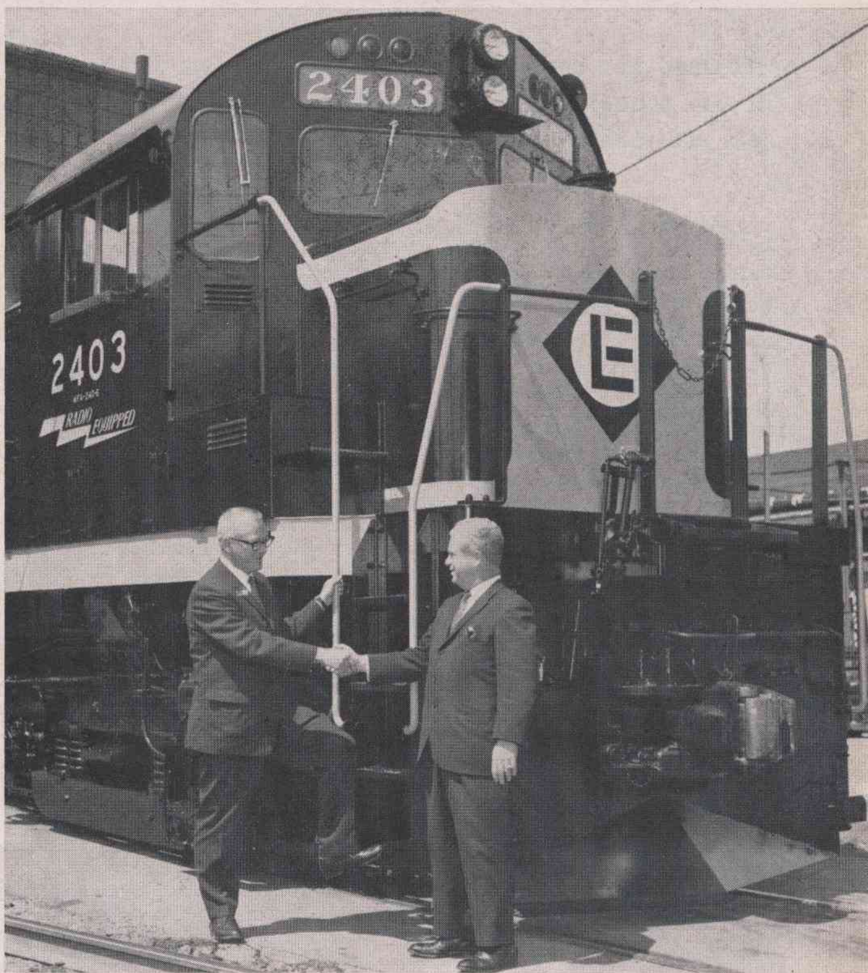
FIRST ALCO CENTURY LOCOMOTIVE is shown during inspection by W. G. Carlson, chief mechanical officer, E-L (left) and W. F. Lewis, executive vice president, Alco. The 2,400-horsepower unit has a pressurized engine compartment.
