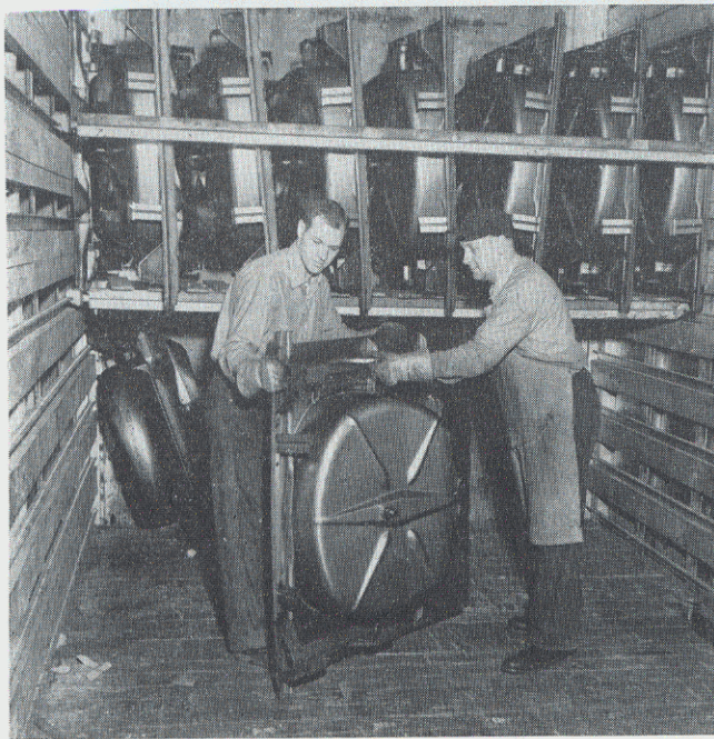
LARGE TRUCK PARTS are handled in cars which allow each unit to rest in its own crib. The Erie provides specially designed cars such as these.
