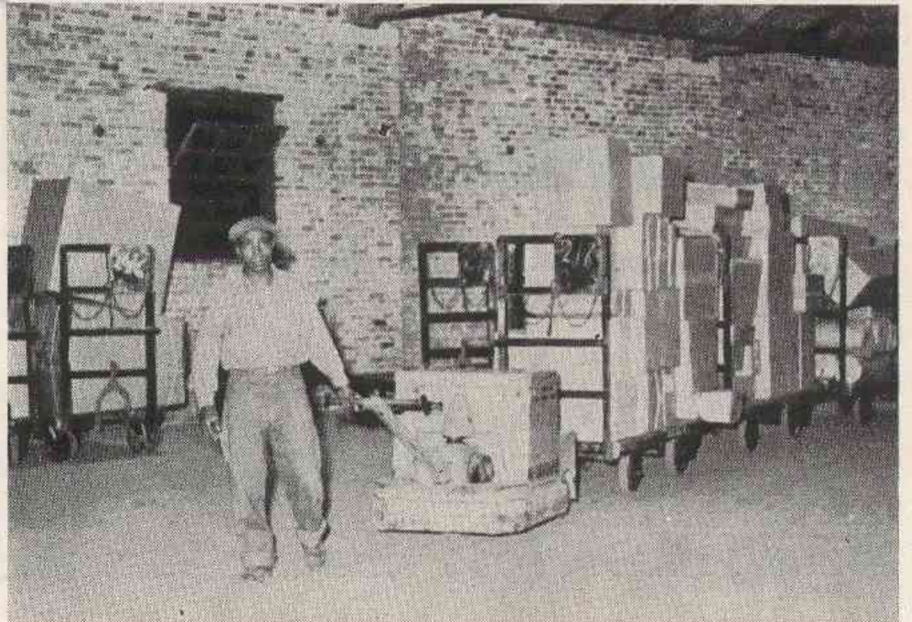
LOADED HOUSE TRUCKS move from the "fingers" to designated zone areas on the second floor. Yale work-savers, called "walkies," are used since there is no Towveyor on this floor.
