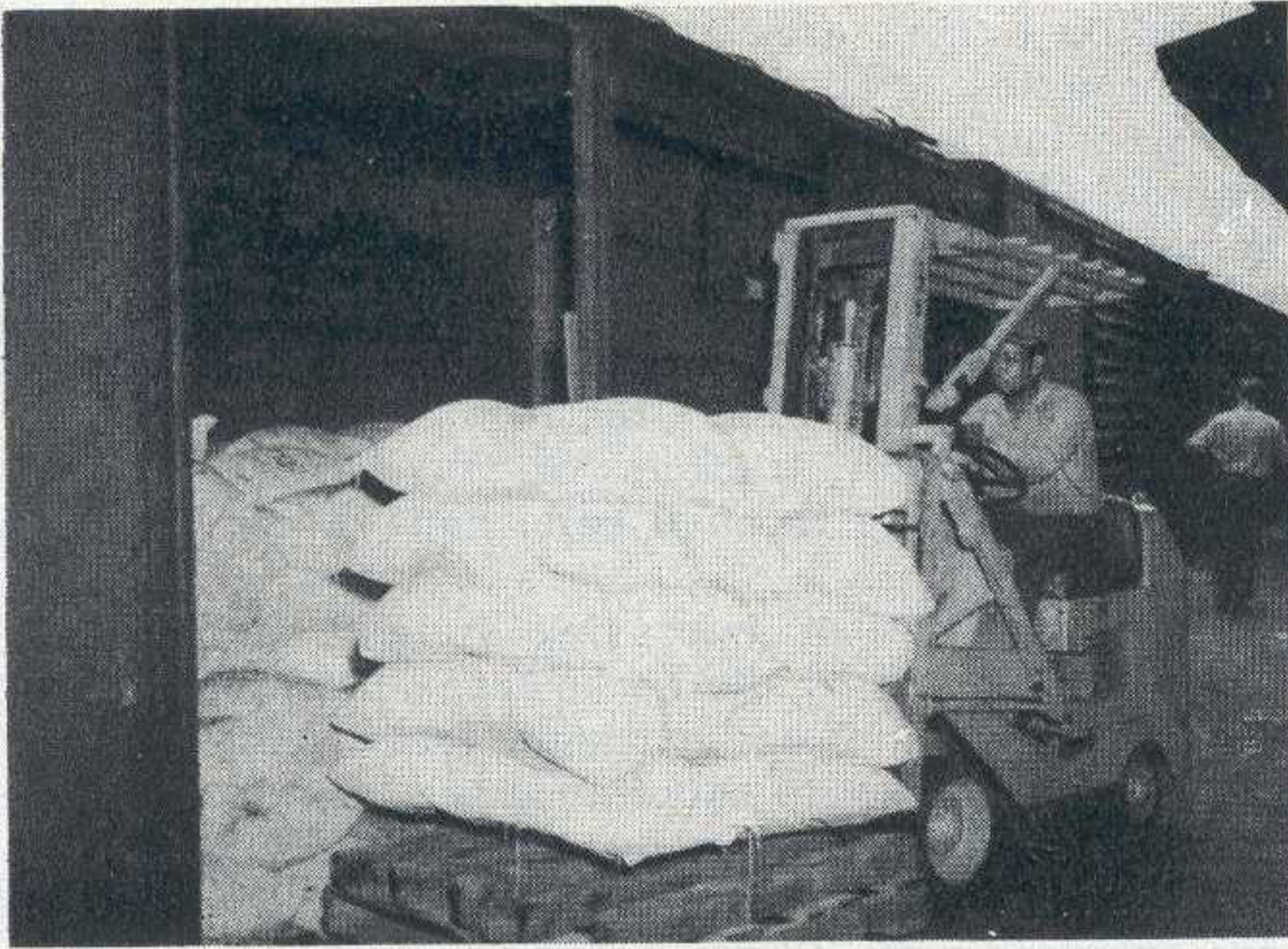
Fork truck, equipped with push-off device, picks up load of sugar from take-it-or-leave-it pallet at Hoboken piers, which have a total of 35 fork trucks
