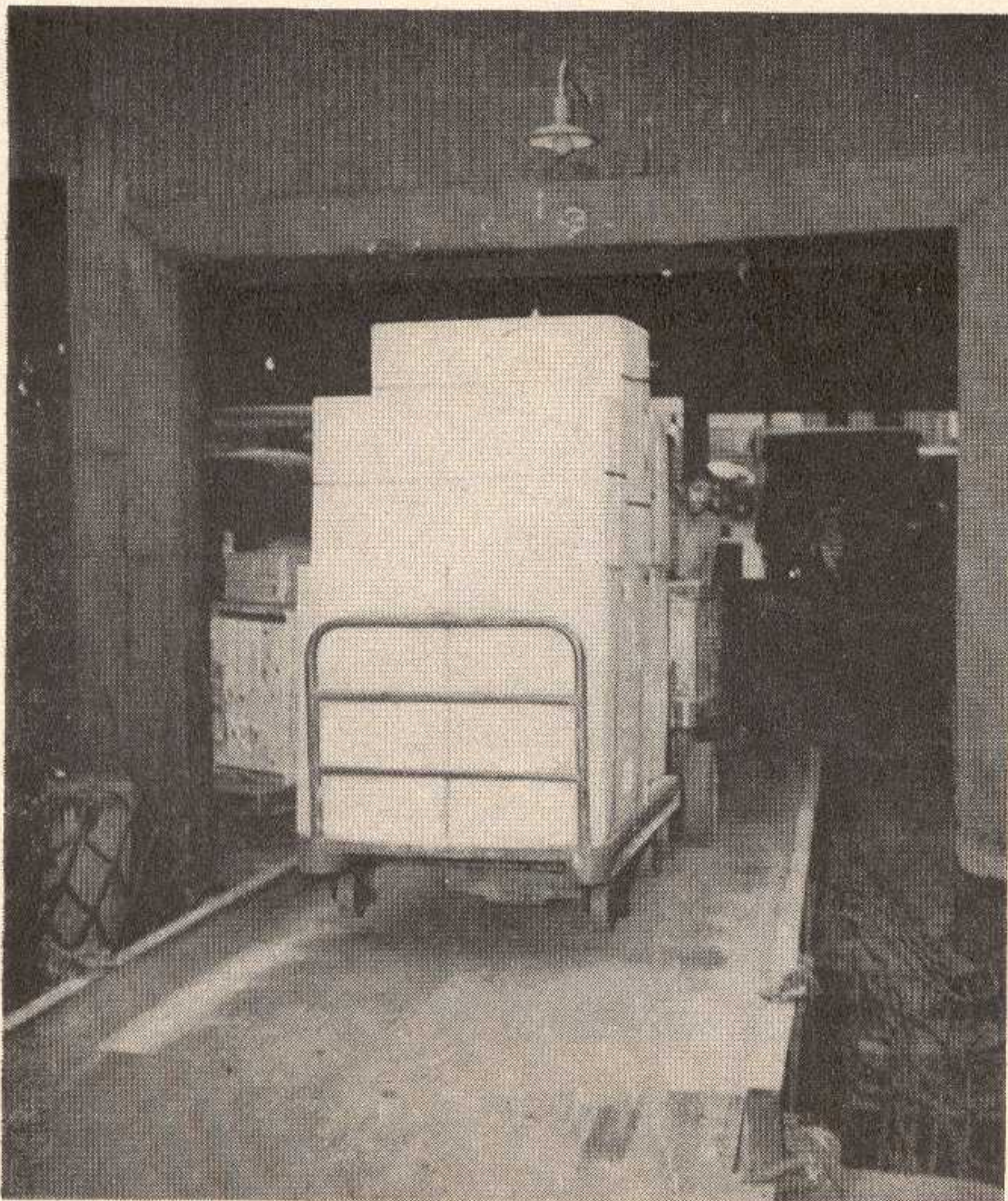
At Pier 68 in New York a low-lift truck takes a loaded live skid up the ramp onto a car float
