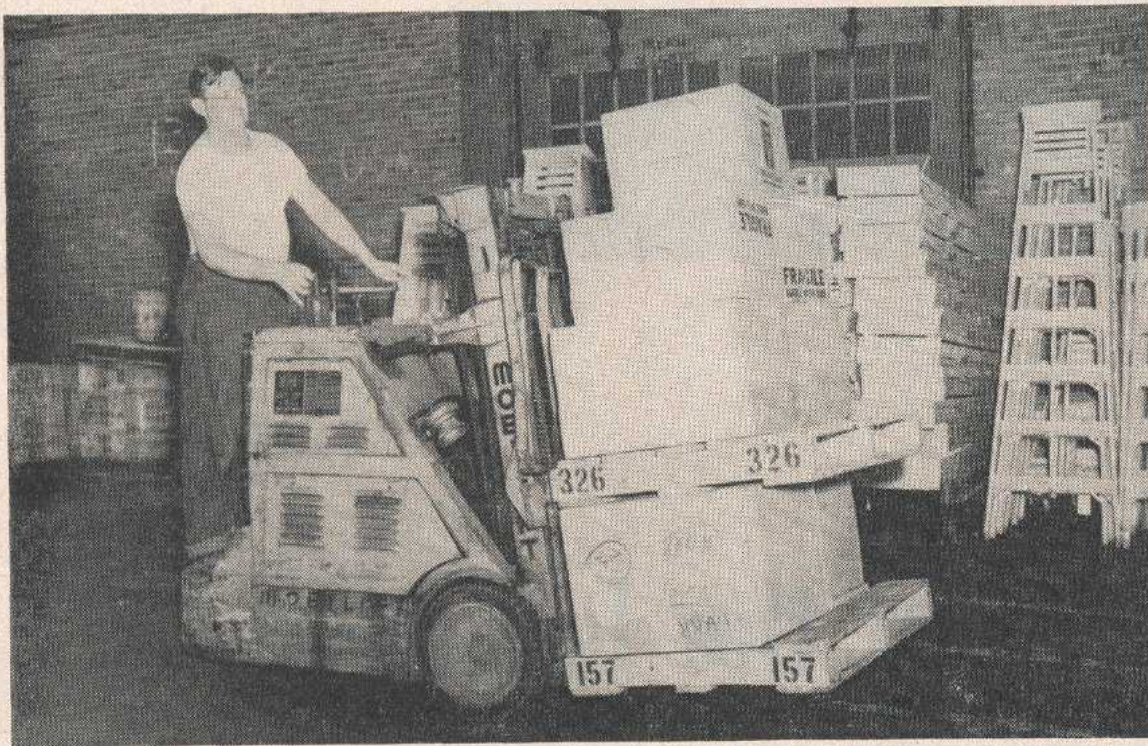
Two pallets loaded with merchandise are being moved at the Passaic, N. J., station by a 2,000-lb. capacity fork truck
