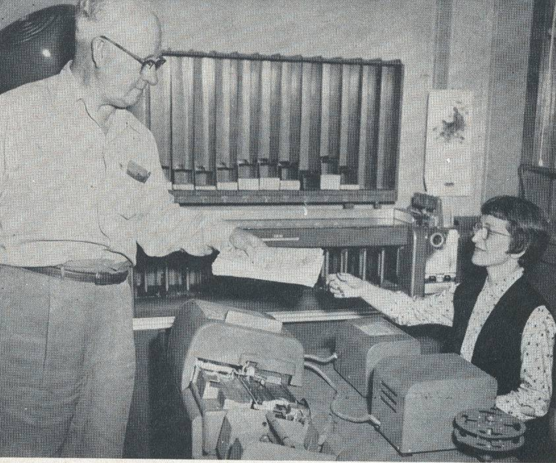
WAYBILLS go to operator who prepares punched cards from them containing pertinent information. Cards then go to . . .
