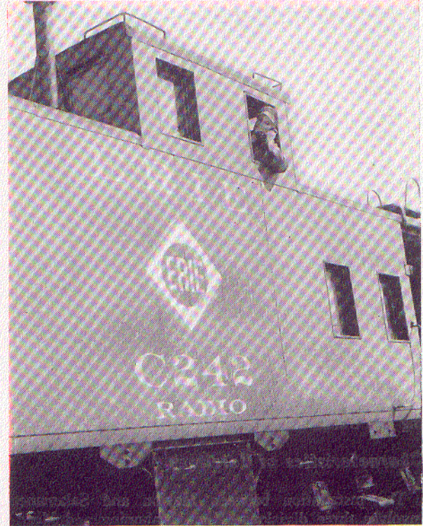
Conductor in cupola of caboose using radio. Storage batteries for operation of the equipment are located in the battery box under the floor
